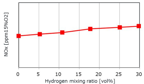
Fig. 10 NO<sub>x</sub> with respect to hydrogen mixing ratio
