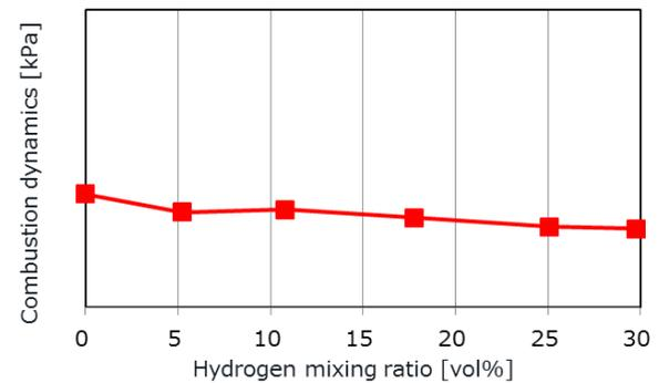
Fig. 11 Combustion dynamics with respect to hydrogen mixing ratio
