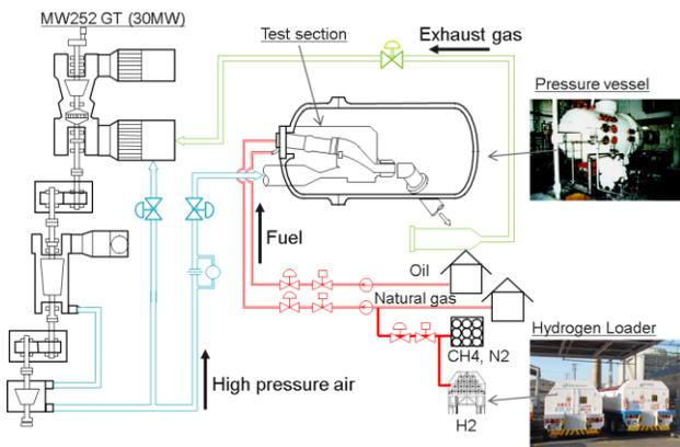
Fig. 9 Configuration of actual pressure combustion test equipment
