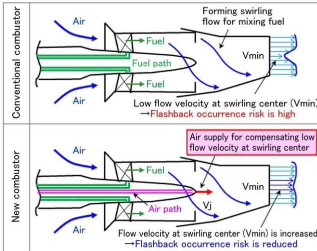
Fig. 6 Outline of conventional combustor and new combustor
